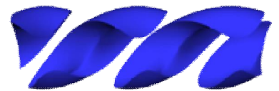
Profile of the Cavity between the rotor and stator
